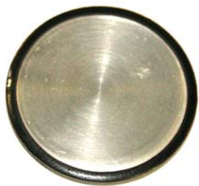
Figure 1a. 30mm Power Diode Pellet
