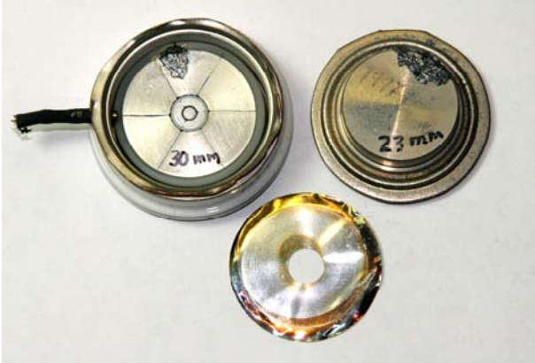
Figure 3. 30mm Power Thyristor Pellet and Case
